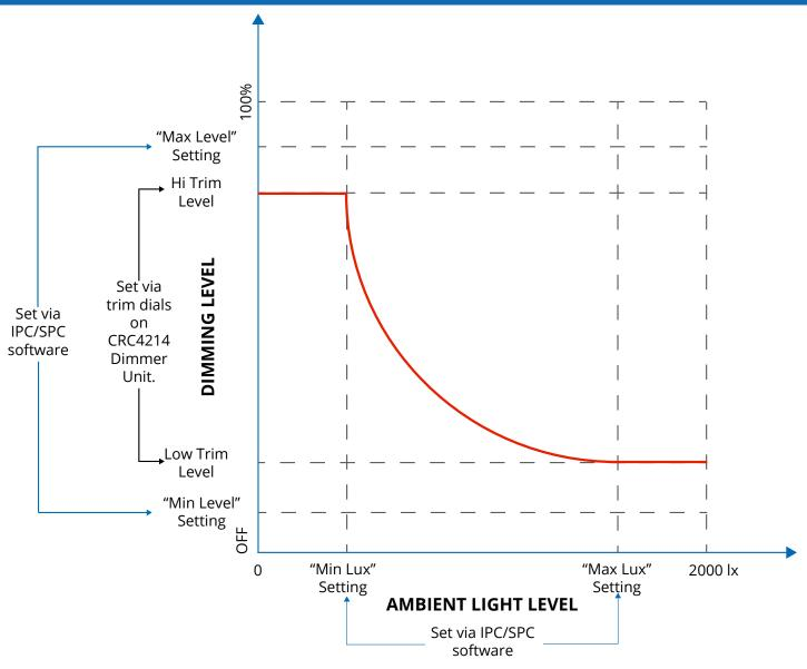
Using the Sensor Dimming Setting Menu on the IPC/SPC:
